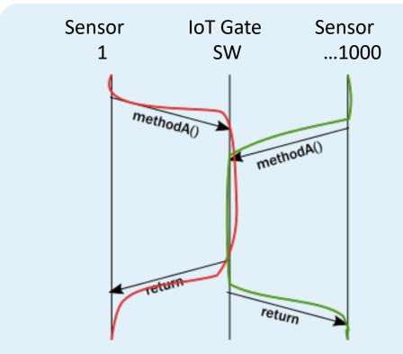
Locking based approach. Only one sensor execution thread can access Gate object at time. This makes CPUs idle. Data harvesting is not real-time and slow.
